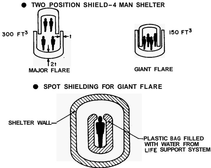
Figure 7. Concepts for Reduced Solar Flare Shield Weight
