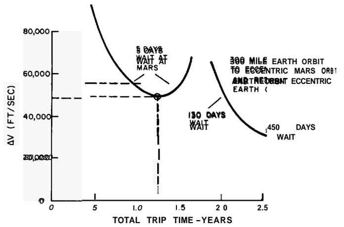
Figure 14. Mars Velocity Requirements for 1971 Departure
