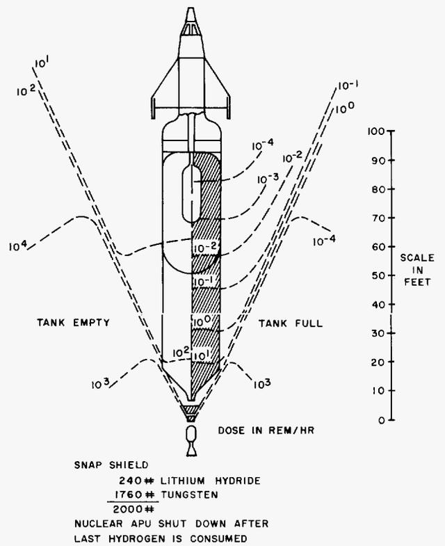
Figure 10. Isodose Plot for 8Kw Nuclear Thermoelectric APU
