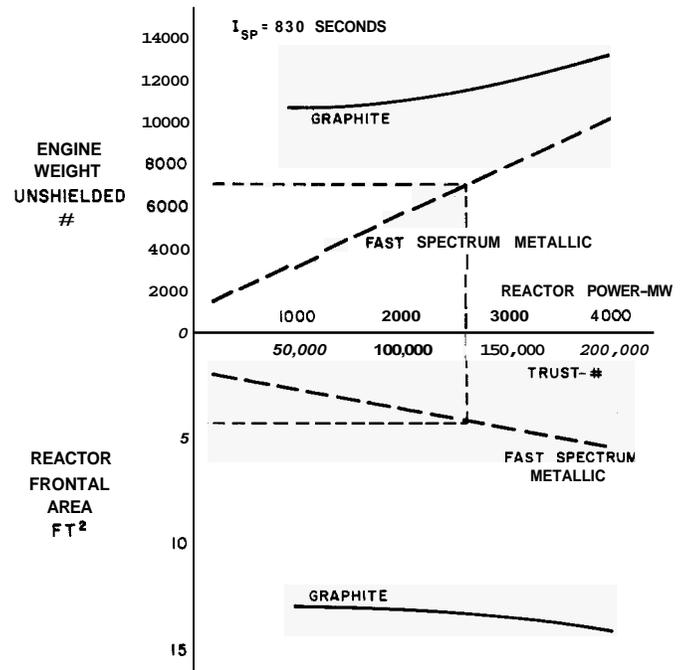
Figure 16. Nuclear Rocket Engine Size and Weight
