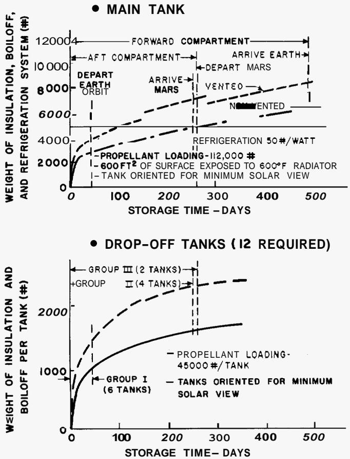
Figure 24. Weight of Insulation and Storage Systems for Liquid Hydrogen Propellant
