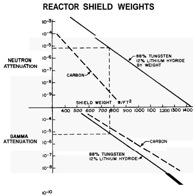
Figure 18. Nuclear Rocket Shield Weights
