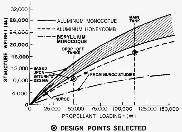
Figure 22. Structural Weights for Liquid Hydrogen Tanks
