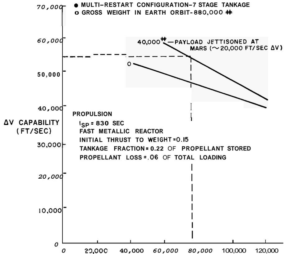
Figure 27. Performance vs. Payload for Multi-Restart Nuclear Rocket Vehicle
