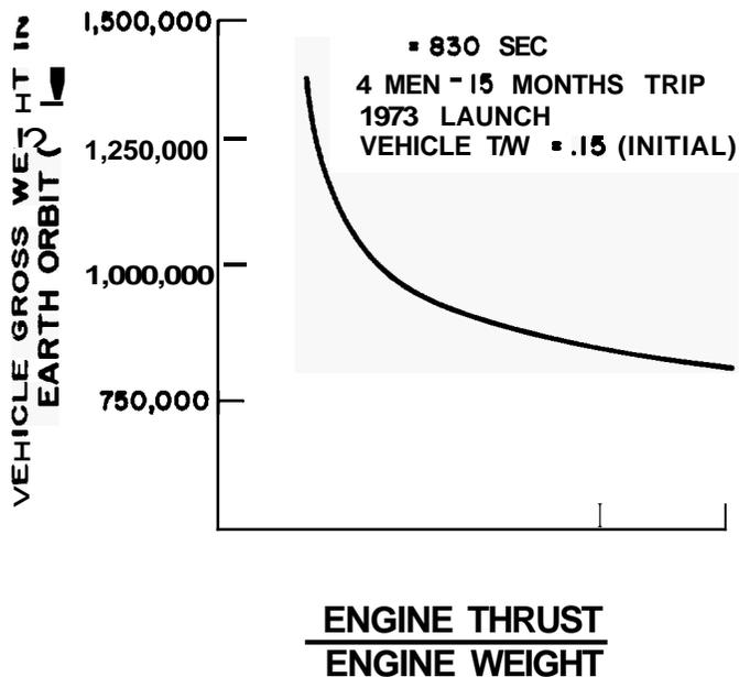
Figure 19. Effect of Engine Weight on Vehicle Weight Requirement
