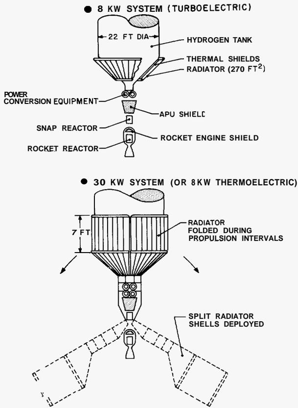
Figure 9. Integration of Nuclear Electric APU
