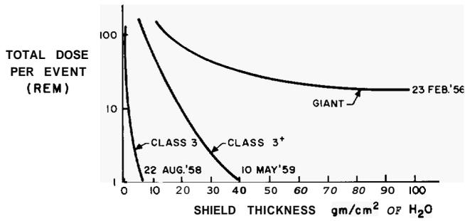
Figure 5. Solar Flare Shielding Requirements
