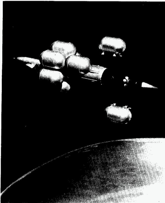
Figure 3. Staging of Propellant Tanks During Earth Escape
