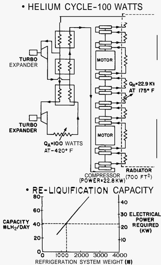
Figure 23. Cryogenic Refrigeration System Characteristics
