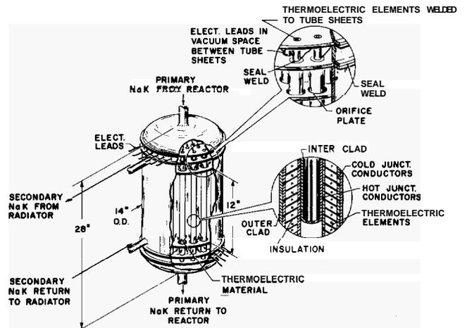
Figure 8. Thermoelectric Generator Arrangement
